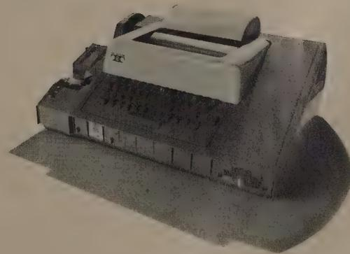
With a built-in paper tape reader and punch and hard copy output, this *ASR-33 Teletype* is perhaps the most versatile of all low cost input/output devices.
