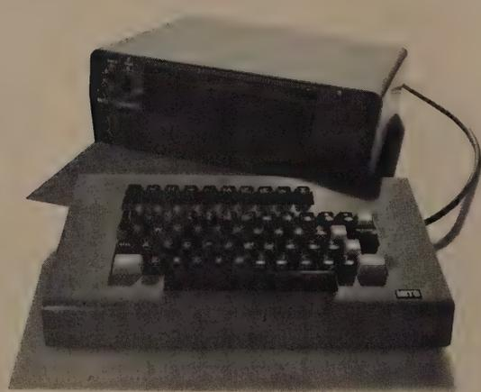
The *Comter II* is easily the most advanced computer terminal kit on the market. It has its own internal memory of 256 characters which combines with a highly-readable, soft orange 32 character display to provide ease of operation and information retrieval.
